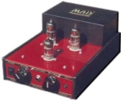
*Ear+* - By using the Hammond 119DA output transformers, bass response was extended down to 10 Hz flat! The output impedance was 7 Ohms! The first production units had both volume and balance controls. Some had preamp outputs taken from either the first stage (5751) or the cathodes of the output tubes.
