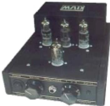
*Ear++* – By adding an output buffer stage (12BH7A), low impedance line outputs were again offered along with two switched line inputs and, in the latest *Ear++ II*, individual channel level controls for balance and overall gain adjustment.
