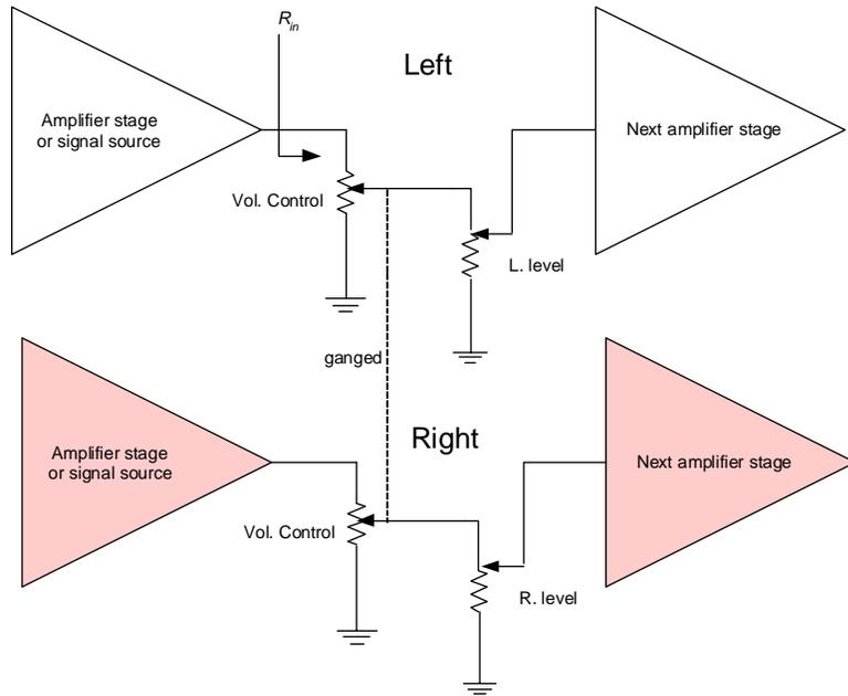
Individual channel level controls in cascade with a ganged volume control. The level controls are shown at their normal (zero attenuation) positions.
