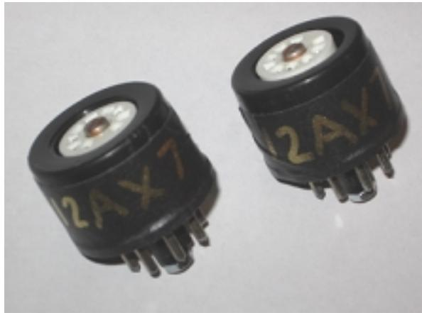
The main variants you can try with these adaptors are the 12AX7A, ECC83, 5751, and 7025. Other 12 V dual triodes that have the same pin connections can be used as long as the heater current is no more than 0.15 A per tube.
