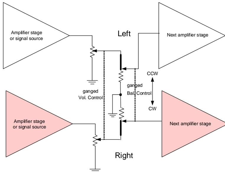
A specially designed ganged potentiometer balance control. There is no attenuation of either channel at the mid position.
