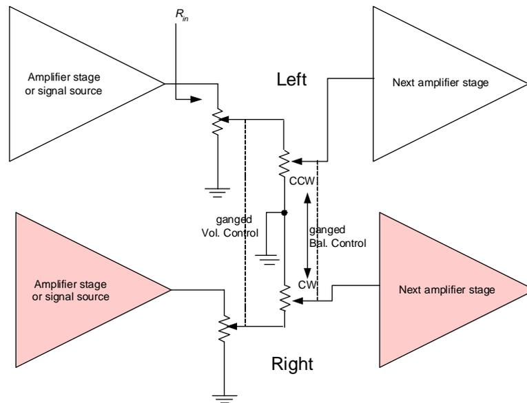
Ganged potentiometer balance control with 6 dB attenuation at mid position.
