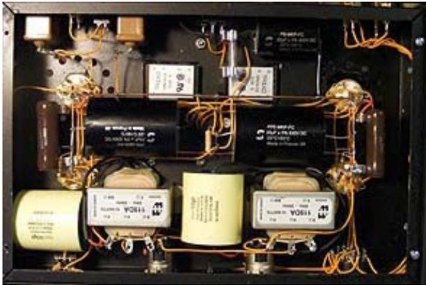
Note the size of the 33  $\mu$ F Auricap output capacitors!
