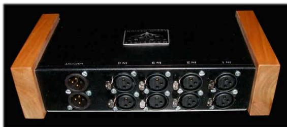
A hybrid router with both balanced and single-ended signals requires a balanced to single-ended conversion if input and output signals are not of the same type. This requires connecting the + signal of the balanced connection to the reference pin to produce a single-ended signal equal to just the + signal. If phase inversion is desired, the + signal can be connected to the reference instead. Here is the required wiring for a non-inverting conversion at a XLR input jack.
