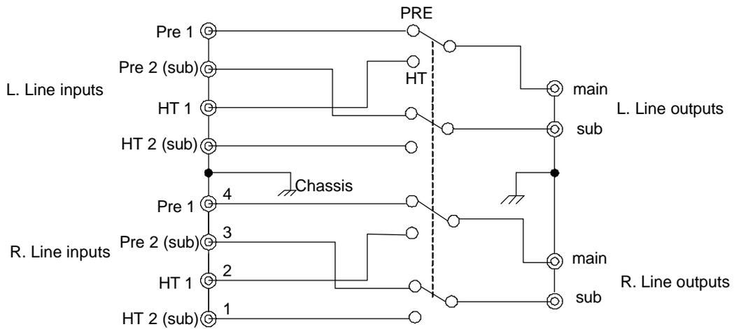
Finally, here is a mode switch modification to control the stereo-mono modes with the mono signal derived from the sum of L and R signals, only L, and only R. Stereo reverse is also available. The position of the Mono switch only affects the output in mono mode.
