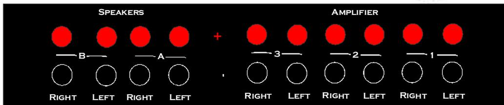
Top – A 3-amplifier to 3-speaker systems *SP 1*. Functional wiring diagram is shown on top of chassis. Bottom – Rear panel layout of a 3 to 2 *SP 1*
