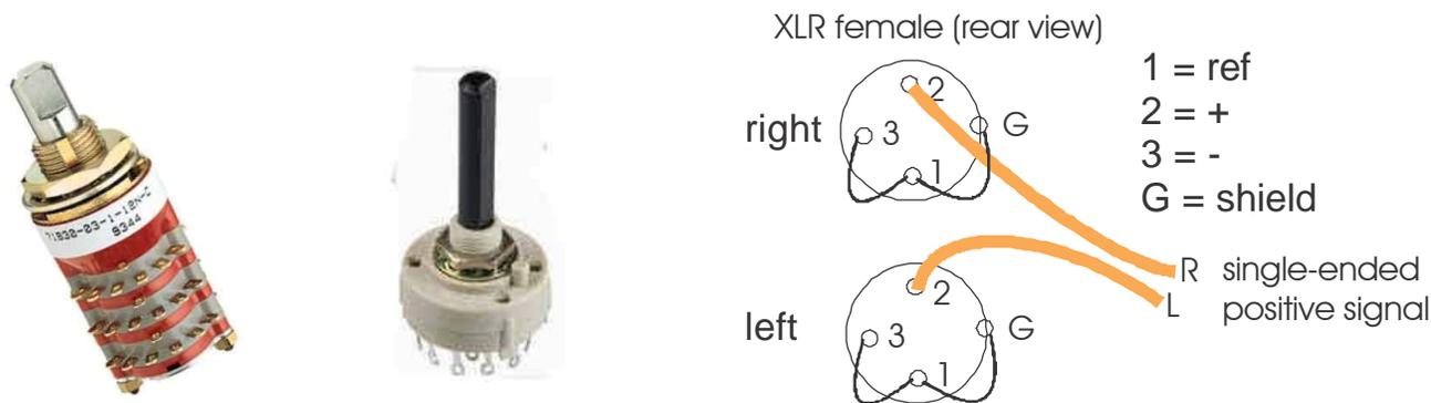
L – Grayhill multi-deck rotary switch, R – Standard Lorlin (U.K.) rotary switch
