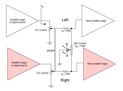
A signal steering balance control. With the values shown, there is a 6 dB attenuation of both channels at mid position.
