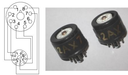
The main variants you can try with these adaptors are the 12AX7A, ECC83, 5751, and 7025. Other 12 V dual triodes that have the same pin connections can be used as long as the heater current is no more than 0.15 A per tube.
