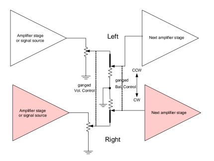
A specially designed ganged potentiometer balance control. There is no attenuation of either channel at the mid position.
