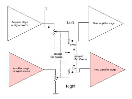
Ganged potentiometer balance control with 6 dB attenuation at mid position. The input resistance is constant but signal levels see-saw.
