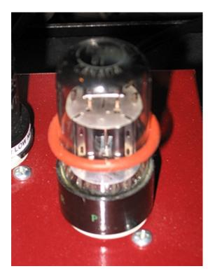
"O" rings have been used as tube dampers with some success in the past. A great source of very soft rubber rings is available every time you replace a headlight in your car. The red "O" ring gaskets can be rolled out of the socket over the lamp and are perfectly sized for a glass octal-based tube.
