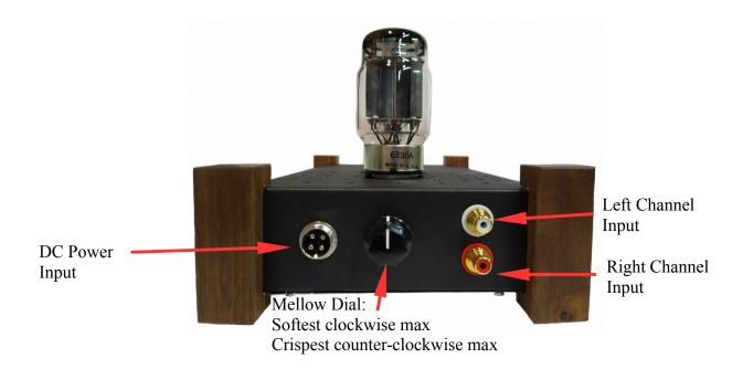
The Mellow Dial at the rear of the amplifier unit is to control the softness of the of the music being played. Softest is when the dial is rotated completely clockwise and crispest when completely counter clockwise.
