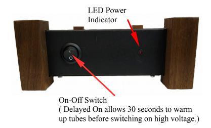
The power supply is connected to the amplifier chassis with the supplied power interconnect cord. Never power on the power supply without making this connection. The two chassis may be stacked or separated as permitted by the power interconnect cord.
