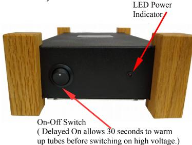
The power supply is connected to the amplifier chassis with the supplied power interconnect cord. Never power on the power supply without making this connection. The two chassis may be stacked or separated as permitted by the power interconnect cord.
