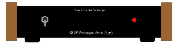
The Mapletree Audio Design *PS 2D* power supply provides +12 VDC (regulated) heater supply voltage and +200 VDC B+ plate supply voltage at a current of 15 mA (see specifications). It utilizes low-noise ultra high-speed diodes to achieve low noise with the high efficiency of the bridge rectifier topology.
