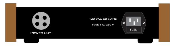
Once the interconnecting power cord is securely attached between the two chassis and the line cord is plugged in, the power supply can be turned on. The pilot lamp on the power supply chassis indicates that the unit is on. It takes about 30 seconds for the tubes to reach operating temperature ready for use. During operation, is it normal for the power supply chassis to become warm to the touch.
